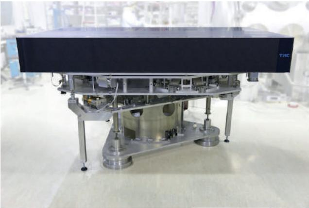
A single-stage solution is available and provides 40 dB suppression of seismic motion in all six degrees of freedom. It is available in a vacuum compatible configuration and supports a pay-load of up to several tons.
